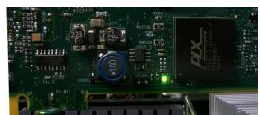
Figure 1: 8xGTe powered on and communicating (D2002 is green)
